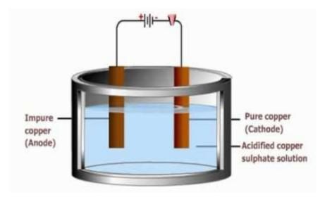
Impurities such as gold or silver fall to the bottom of the electrolytic cell container because:
